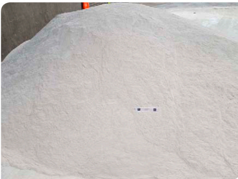
Below: The final product is chemically identical to natural gypsum.
