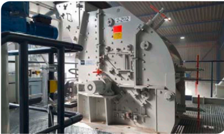
Above: The BHS type PB impact crusher. The combination of shredding and impact crushing produces particularly pure recycled gypsum.
