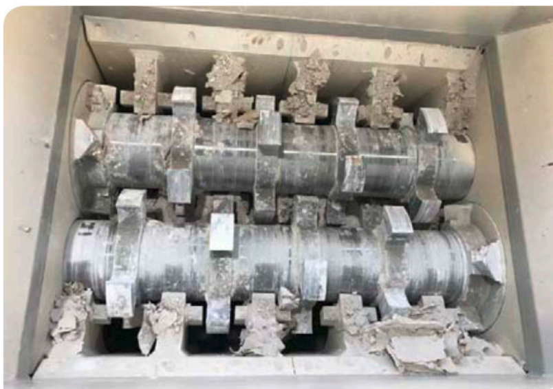
Below: The two shafts of the type VSR pre-shredder are equipped with shredding tools that can easily handle impurities in the gypsum waste.
