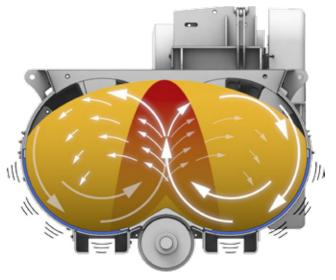
Mixture movement and pulsating rubber trough of the DKXK
